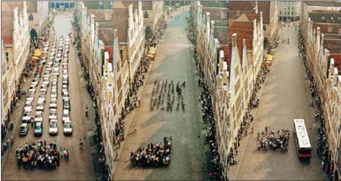
Figure 3.12: Road space required by 50 people driving cars (left), motorcycles (center), and riding in a bus (right)
