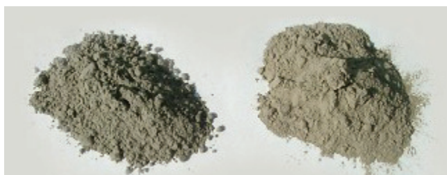
Figure 12: Cement (on the left) and fly ash (on the right) look very similar
