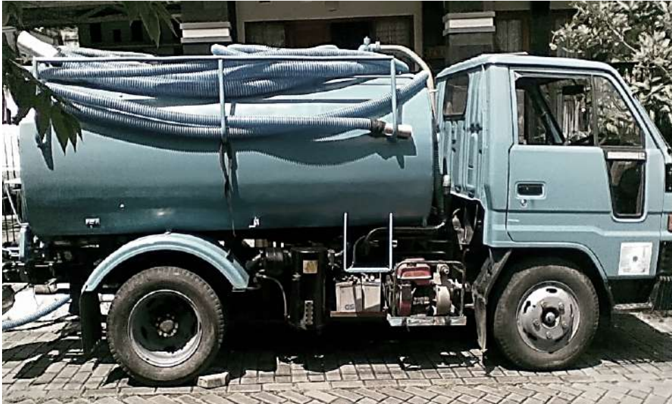
The most important parts of a desludging unit are 1) sludge tank, 2) vacuum pump and 3) desludging hose. Each unit must also carry safety equipment and first aid kit box.
