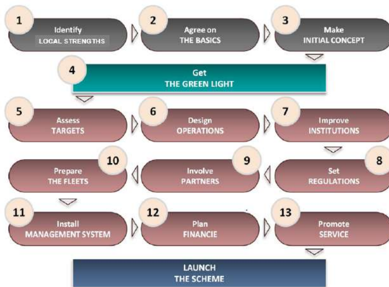
The thirteen generic steps to set up the scheduled desludging scheme in a city.
