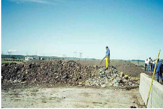
Figure 7 Sprinkling FS over refuse at the Rini/ Grahamstown (South-Africa) co-composting plant
