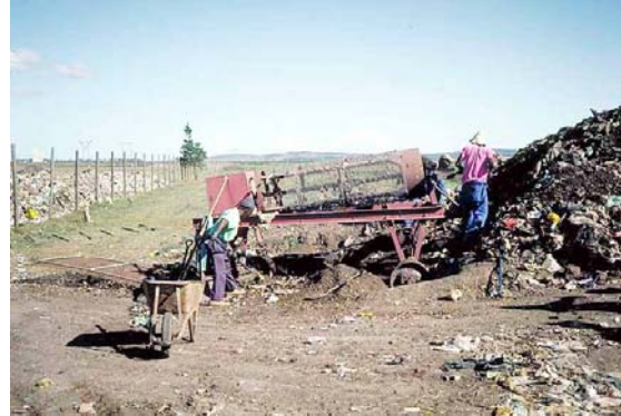
Figure 8 Sieving of matured compost in a rotary sieve at the Rini/Grahamstown (South Africa) co-composting works
