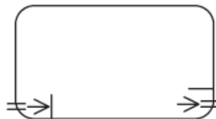
Figure 13: Stub baffles according to Shilton and Harrison
