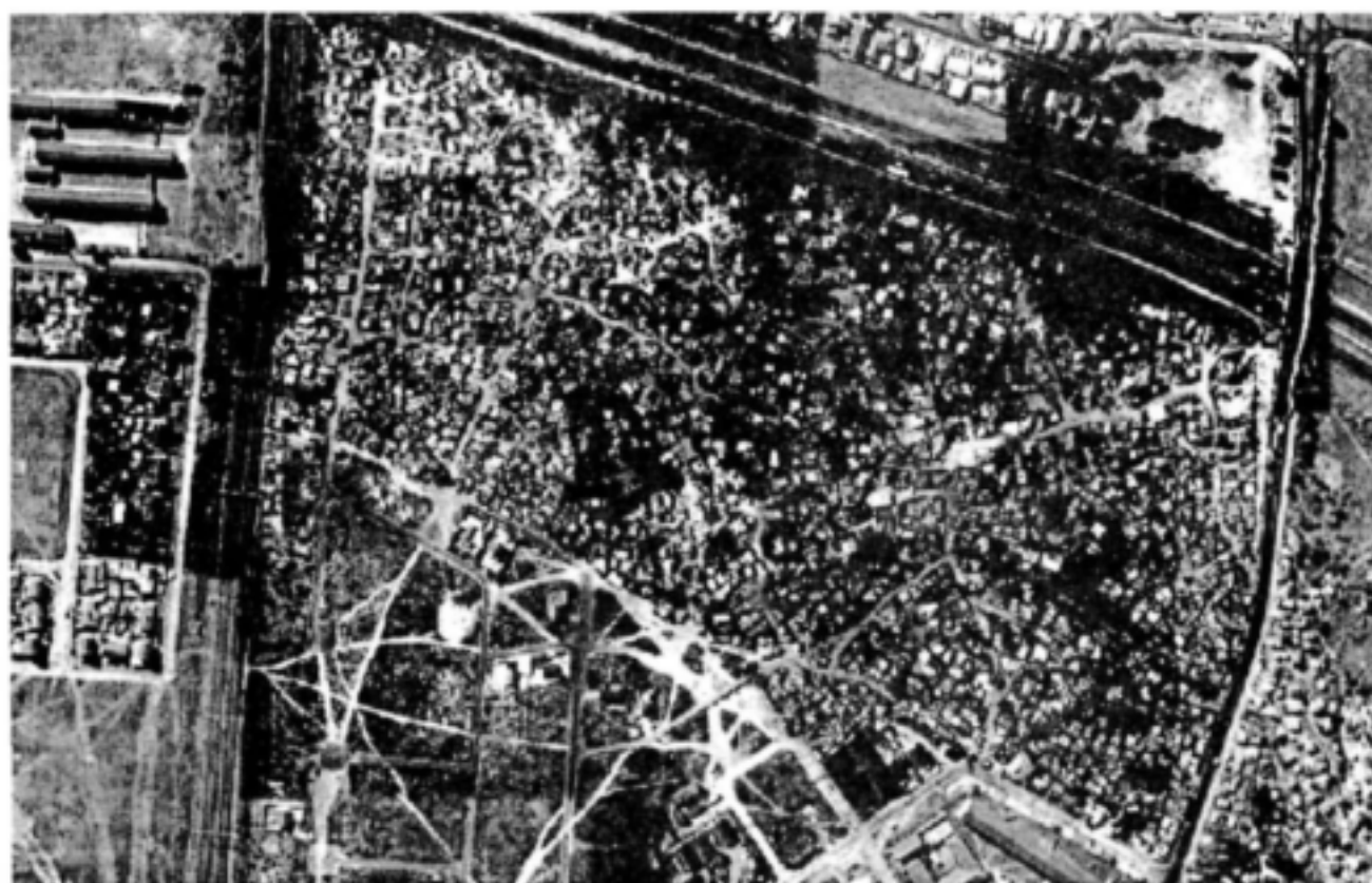
Figure 3.5: Mosaic of warped 1999 helicopter images of New Rest superimposed on a 1996 1:20 000 aerial photograph
