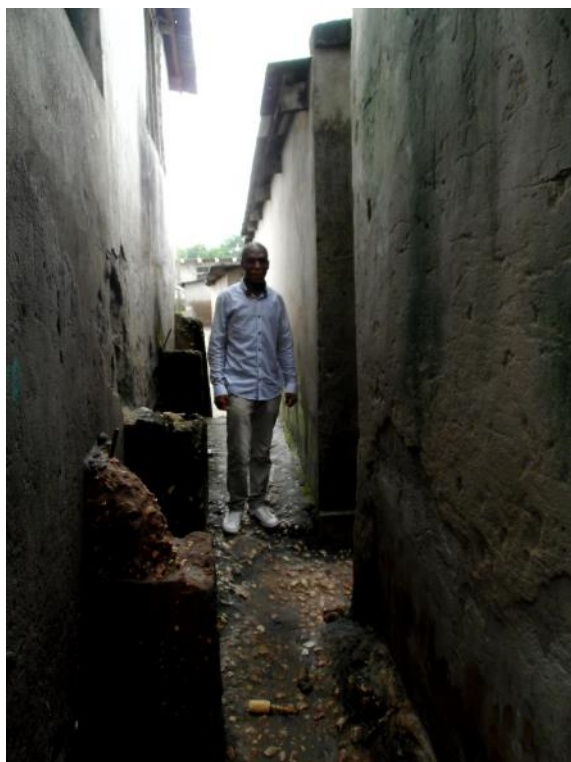
Path inaccessible to vacuum trucks
