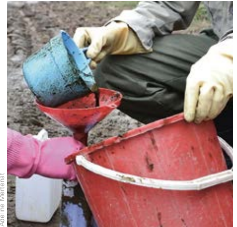
Photo 2: Repartition of the sampled FS into bottles for laboratory analysis.
