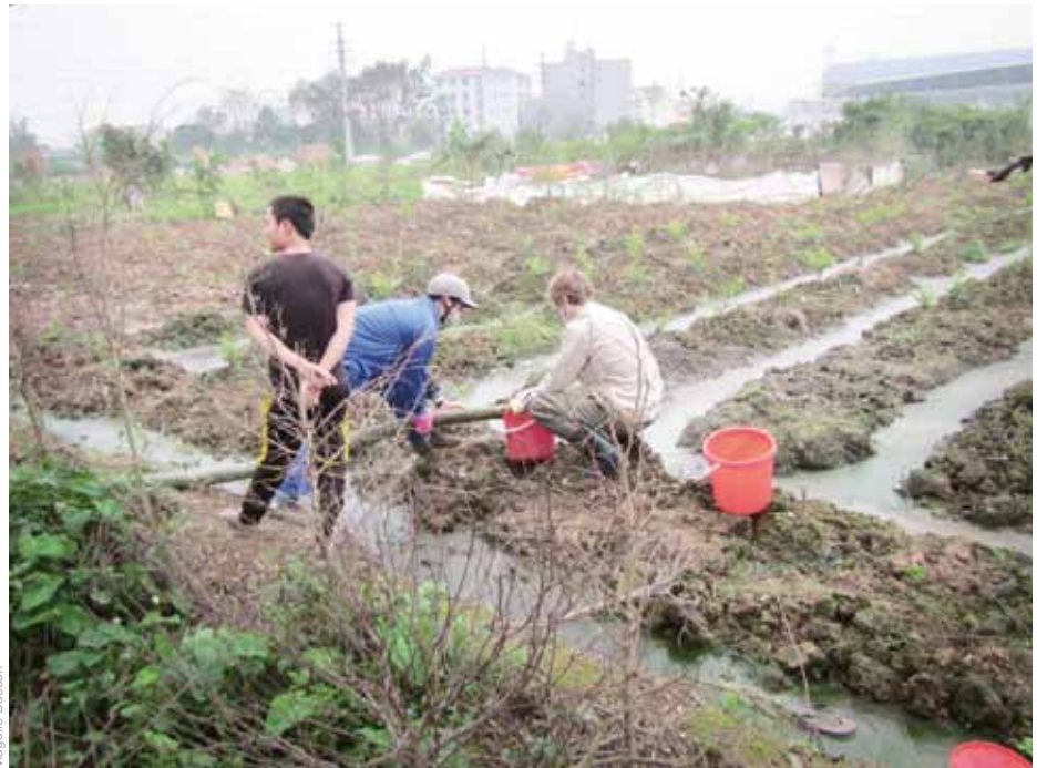
Photo 3: Grab samples being collected at a discharge site.
