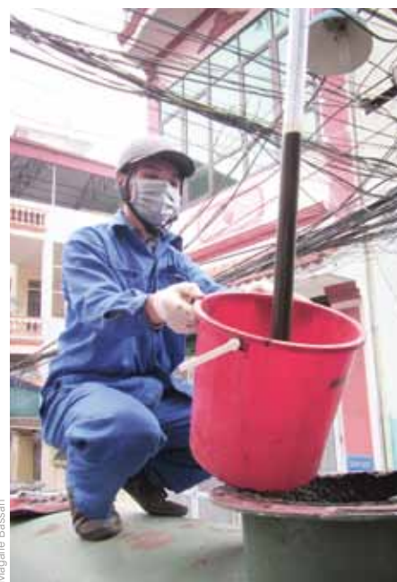
Photo 2: Sampling from the access port at the top of a truck.
