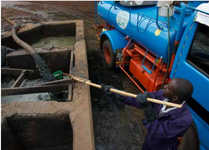
Photo 2. Samples being collected during discharge at Bugolobi Treatment Plant.
