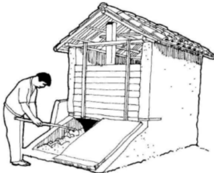
Figure 2.4: A solar-heated dehydrating toilet in Ecuador (Esrey et al 1998)
