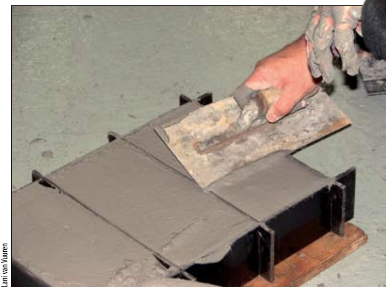
UP concrete technologist Derek Mostert demonstrates the ease of casting foam bricks.
