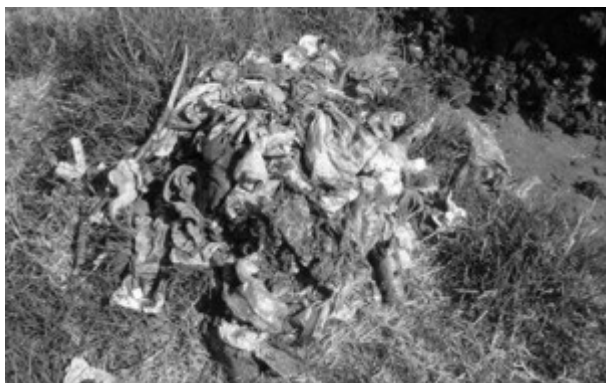
Relatively small amount of solid waste material from exhumed household VIP.
