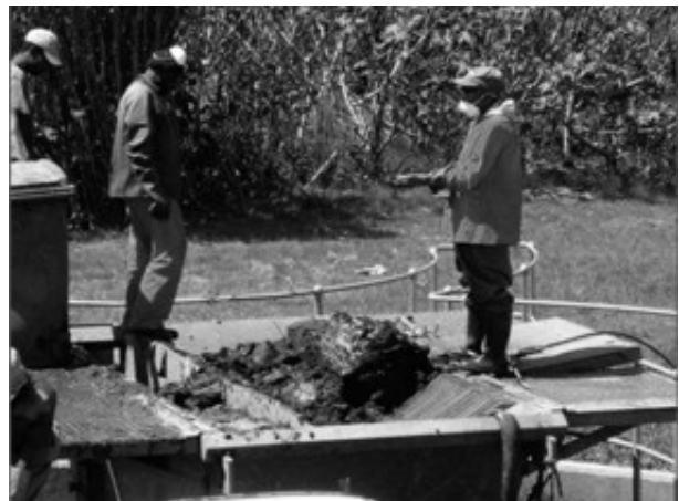
Converted skip with grids for separating solid waste from faecal sludge. Separation is achieved with the assistance of high pressure water spraying
