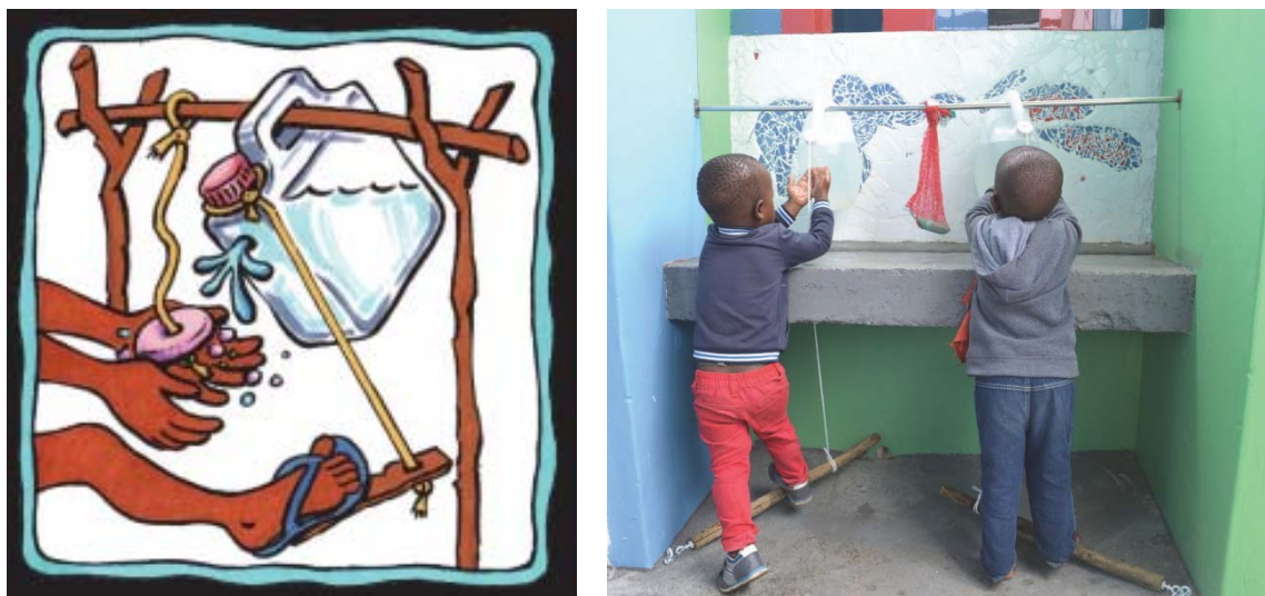
Figure 16: The tippy tap concept explained (left) and in use at a preschool toilet facility designed by Lima/Save the Children in KwaZulu-Natal (right)
