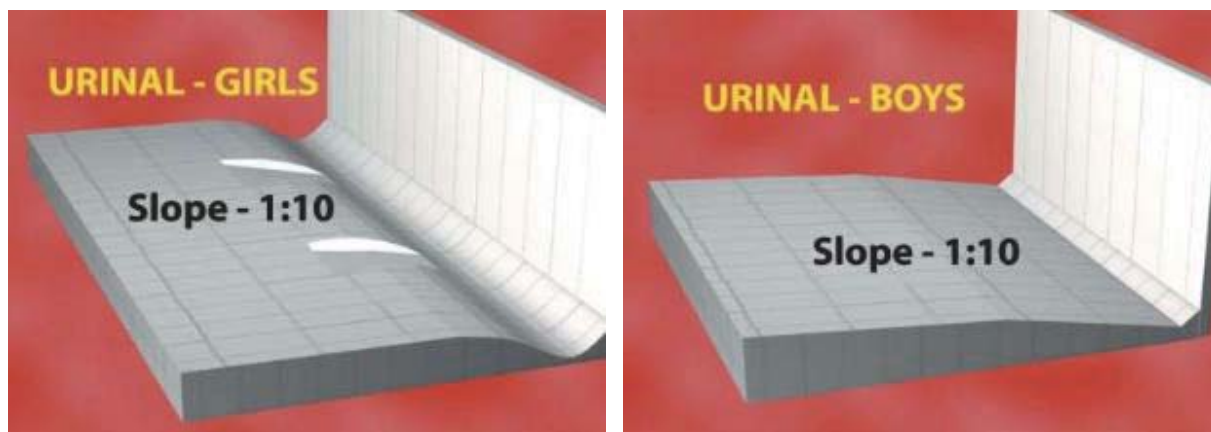
Figure 10: Designs for girls and boys urinals recommended by the Government of India
