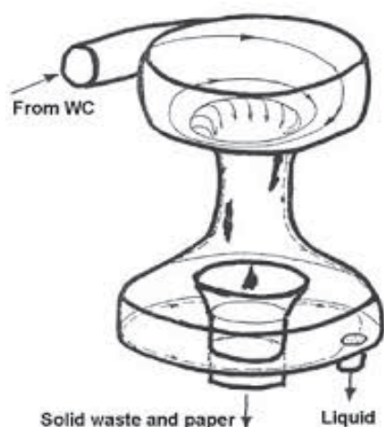
Figure 24: The Aquatron separator which uses a cyclone principle to separate solid and liquid waste
