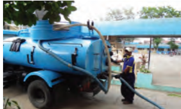
Vacuum trucks for septage collection (Source: Josie Antonio)
