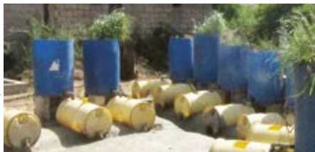
Photo 1: Barrels used for planted drying bed trials (Cambérène Faecal Sludge and Wastewater Treatment Plant).
