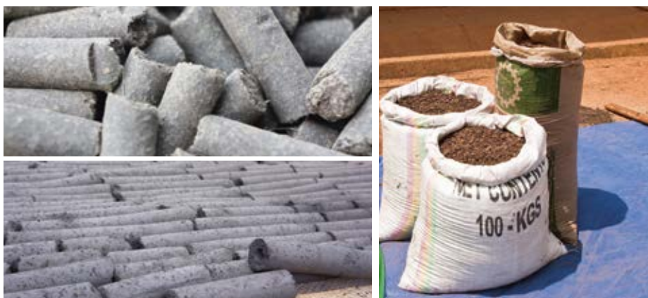
Photo 1: Pellets (top), briquettes (bottom) and crushed fuel produced from FS (right).
