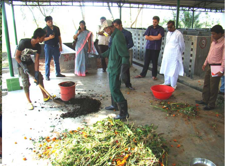
Faecal Sludge Collected by Vaccu-Tug and Discharged in the Drying Bed and later Co-composted with Organic Waste to Produce Compost
