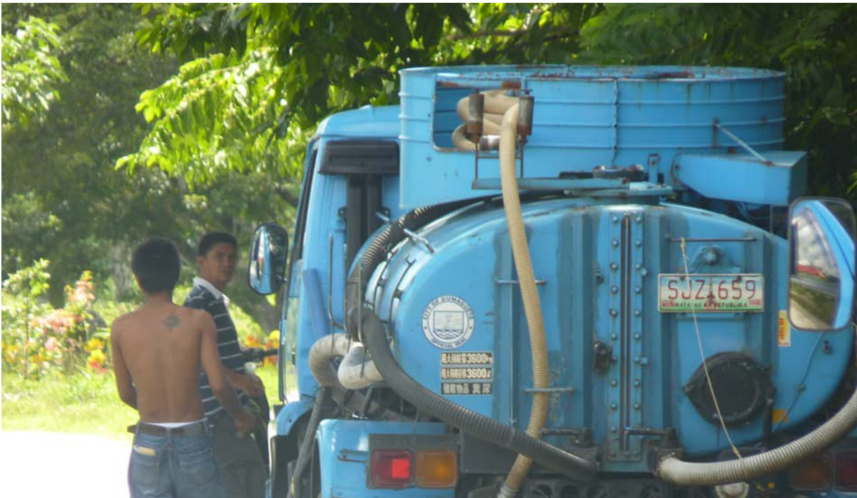
Figure 18. Traditional vacuum trucks. The tanks shown here have a 2.5 cubic meters capacity. Vacuum trucks are available in sizes in sizes from less than 1 cubic meter to up to 10 cubic meters of capacity.
